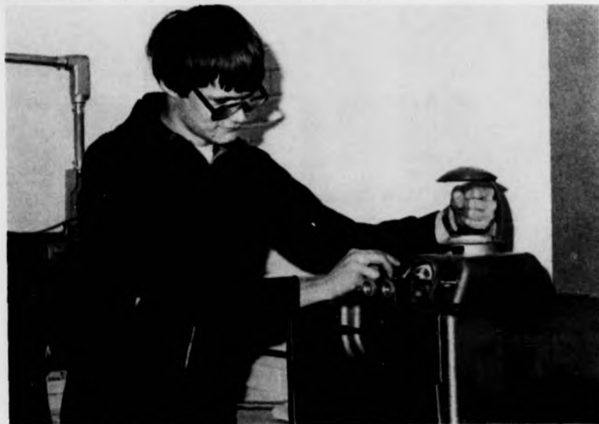
Paul Brown, auto maintenance student, cleans a spark plug in the shops new spark plug cleaning machine.
